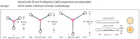
Aluminium structure with three light heads. Each light head can be taken off and is fully adjustable
