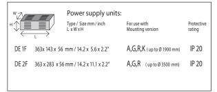
Input voltage for all external power supply units and canopy is 220-240 VAC 50-60 Hz
