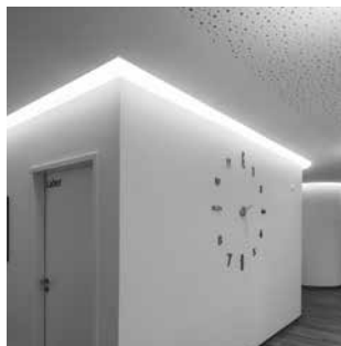
HINTERLEUCHTUNG ●●●●●● COVE LIGHTING | 1020 - 3020 mm | 18 W/m CRI > 90
